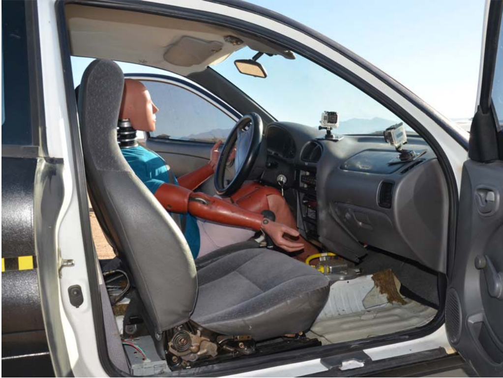
FIGURE 57. Post-Test View of Passenger's Side Occupant Compartment
