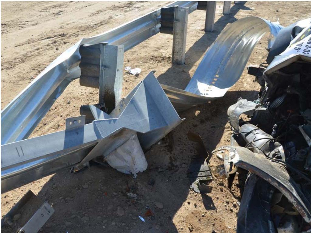
FIGURE 36. Test Article Damage
