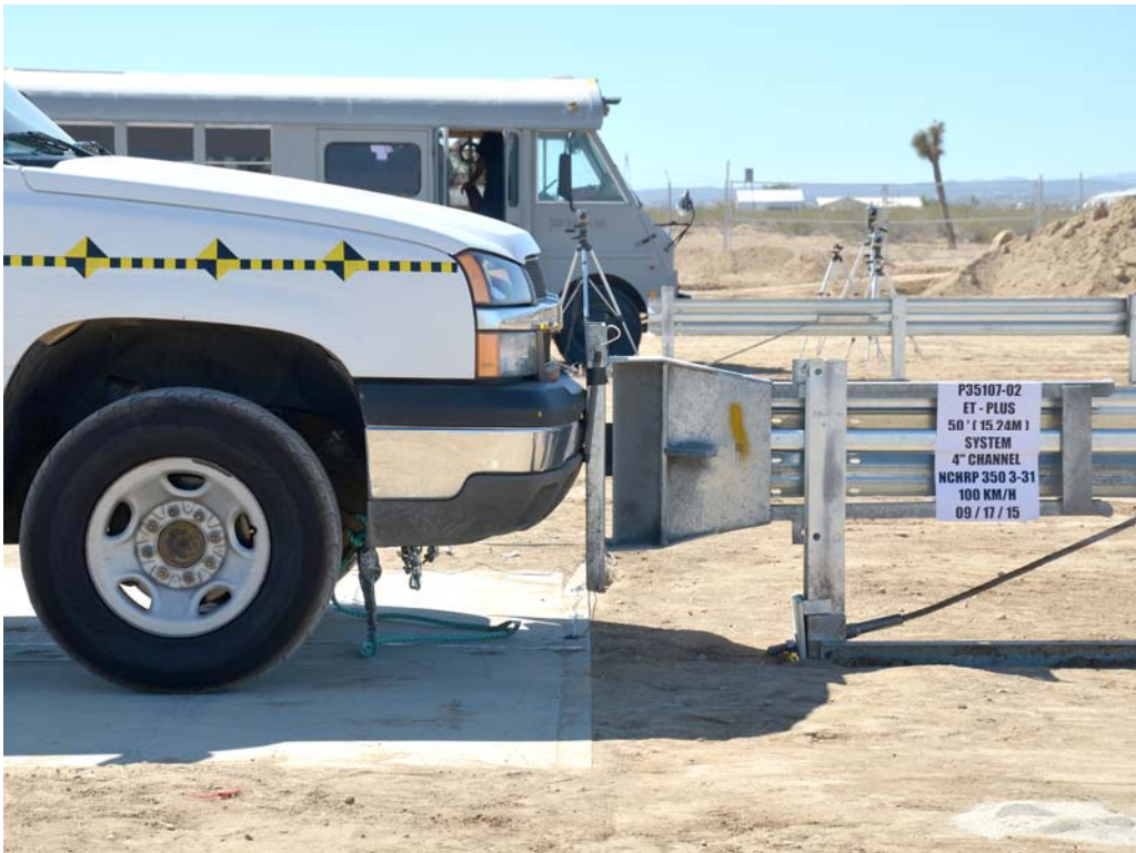
FIGURE 14. Test Setup Close-Up
