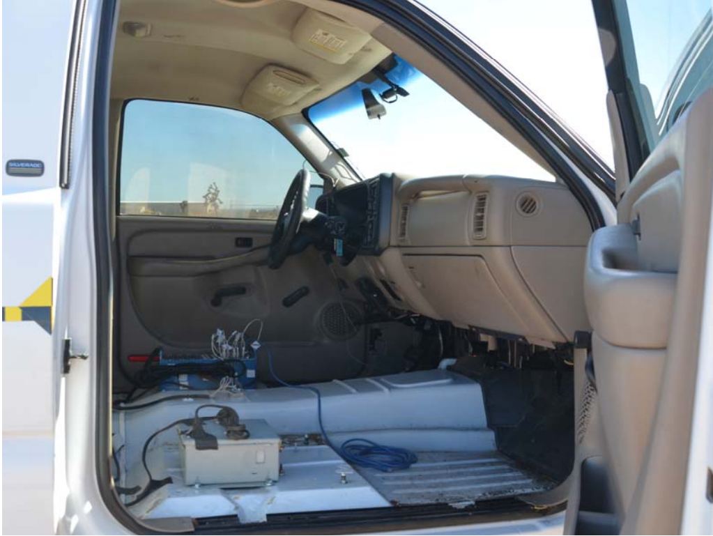
FIGURE 57. Post-Test View of Passenger's Side Occupant Compartment
